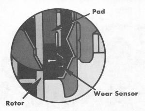
**Front disc brakes** • Resist fade • Recover quickly from water immersion • Lining wear sensor sounds audible signal when pads need replacement.
