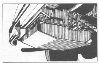
**Shield plates** • Help protect fuel tank over rough terrain • Include transfer case shield plate.
