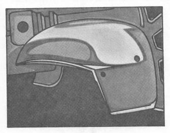
Full front wheelhousings • Protection from stone damage • Ward off corrosion-causing road splash • Self-washing.
