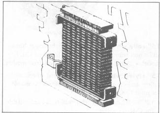
**Engine oil cooler** • Supplements normal cooling through oil sump and engine block • Recommended for heavy-duty trailering • Available only with V8s.
