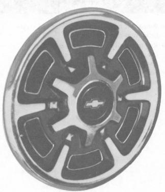
New wheel trim options are available for C/K10 models • A new full black and gray, stainless steel wheel cover in a spoked hub design is available • New optional white-painted wheel features a spoke-type design.
