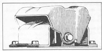
**Engine mount design** • Vibration-absorbing cushion between engine and frame • Front mounts have pre-loaded rubber cushion between steel backing plate and housing to absorb shocks.
