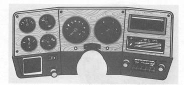
Gauge-type instrument cluster • Provides voltmeter, oil pressure and temperature gauges
