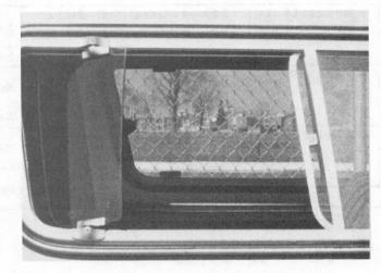
Sliding side window glass • Available with removable plastic hardtop • Replaces fixed side window glass • Improves rear compartment ventilation • Windows have adjustable outboard ventipane sections to control incoming air flow.
