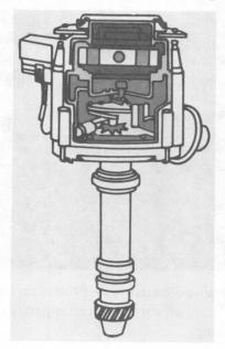
**High Energy Ignition system** • Standard on all engines, Sixes and V8s • Delivers up to 85% hotter spark than conventional systems • Improves cold-weather starting • Provides all-weather protection from moisture, dirt and road splash • Solid-state design eliminates ignition points and condenser, extends the time between recommended tune-ups.
