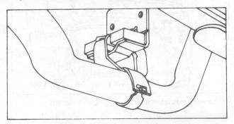
**Compression-positioned exhaust hangers**
