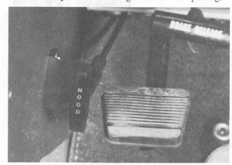
New inside hood latch release • Available for all Blazers • Release handle is on left-hand kick panel beneath instrument panel • Helps prevent theft of underhood items.
