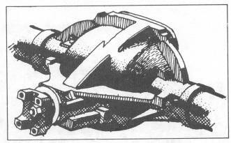
**Salisbury rear axle** • Inherently strong design • Large ring gear, tapered roller bearings, broad ratio coverage.
