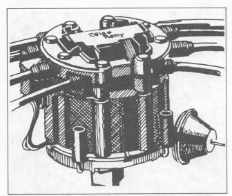
**High Energy Ignition system** • Magnetic pulse generator, electronic control module replace points, condenser and rubbing block • Coil designed for 85% hotter spark than conventional systems.
