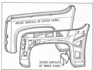
Improved rustproofing • Zinc-rich primer applied to front fender inner and outer panels before welding and final priming • Primer baked on inner surfaces of front door outer panels before forming and final priming • Entire body, doors and tailgate immersed in electrically charged primer.
